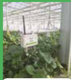
Temperature / Humidity, CO 2 sensor
