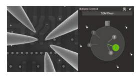
From the main window, the operator is guided through the steps of setting up his nanoprobing system and test recipes, landing probe tips on the device under test, acquiring measurement data and reporting about them.
