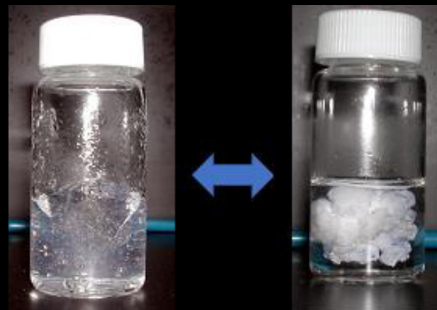
Figure 1. Collapse of Poly(NIPAAm) hydrogel as temperature is increased above 32 °C
