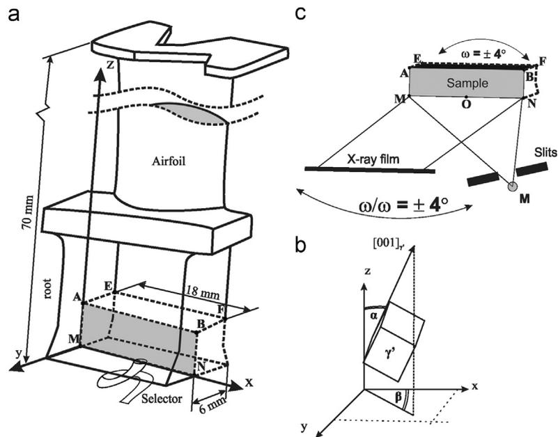
**Fig. 1.** Scheme of the samples location (a), method of determining misorientation angles  $\alpha$ ,  $\beta$  (b) and scheme of obtaining X-ray topograms (c). ABNM—sample surface for investigation (gray); O—the axis of oscillation film and sample; M—X-ray microfocus source.
